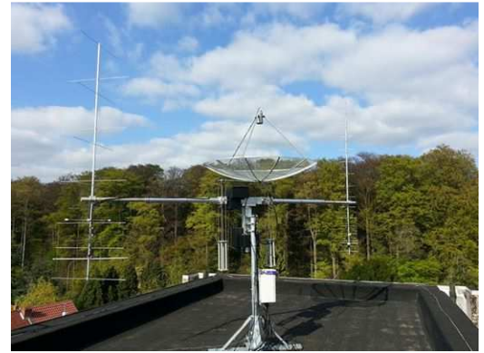
Figure 9: Typical ground station antenna for VHF (left), S-Band (center) and UHF (right). This one is located at the VKI.
